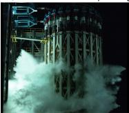
posely pushed a liquid oxygen tank test article to its limits using water to simulate liquid oxygen. The tank test is part of the SLS core stage that produces 2 million pounds of thrust to help launch the rocket. The test ensures the rocket's structure can
